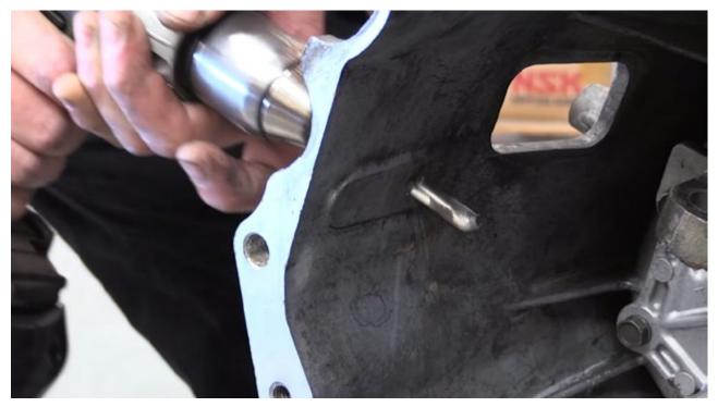
3.) Using an 8.5mm drill bit, carefully drill the first hole for the slave. Ensure that the hole is square to the casting surface.
