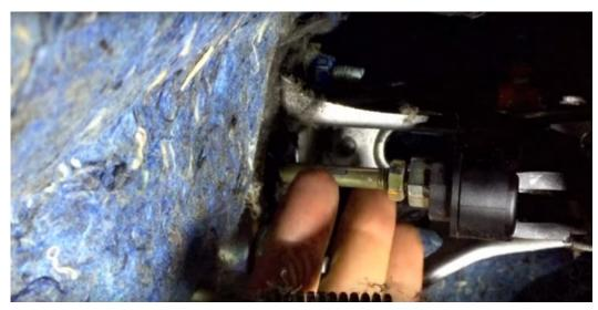
Underneath the vehicle, make sure that the slave cylinder can be depressed by hand and that it 4. pushes fluid back up to the master cylinder. This ensures that the bearing does not hold on to the clutch diaphragm as the clutch wears.
