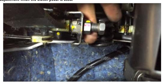
3. Adjust the pushrod from the master cylinder to the pedal by undoing the locking nut and rotating the pushrod. This should still remain slightly free and should be able to be wriggled by hand. This is to ensure that there is no excess pressure on the master cylinder. Tighten the locking nut to ensure that the pushrod does not adjust as the clutch is operated.
