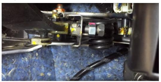
2. Ensure that the locking nut is tightened back against the bracket to avoid unwanted adjustment when the clutch pedal is used.
