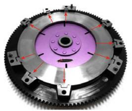
4) Install the top friction disc marked "Gearbox Side" on the intermediate plate.
