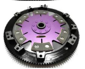
3) Install the intermediate plate over the bottom friction disc. The driving tabs on the intermediate need to index in the flywheel.
