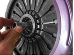
3) Slowly and evenly tighten the pressure plate bolts in the sequence shown ½ turn at a time. Check the alignment of the splines with the alignment tool before finally torqueing these bolts up to 32Nm.
