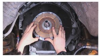
9. Install the main pressure plate casting into the alloy hat with the fulcrum ring facing toward the diaphragm. Slide this over the alignment tool and locate the alloy cover on the flywheel.
