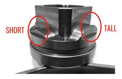
For this kit it is critical to have the lowest contact position mounted against the clutch fork as illustrated below.
