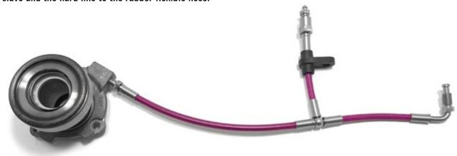
The long section of the hose with the male fitting is threaded into the port on the slave.
