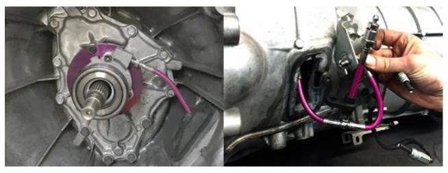
The release bearing and mount can be mounted to the transmission using thread retaining compound on the M6 bolts. The braided line then mounts directly to the original rubber line.
