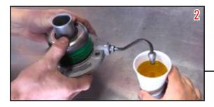
Slowly depress the Slave Cylinder and submerge the line in the fluid.
