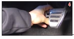
After the transmission has been installed, fill the master cylinder with fresh fluid. Slowly operate the clutch pedal to induce fluid flow from the master to the slave.
