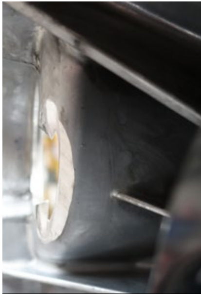
Modified chamfer on the starter pocket from inside bellhousing.
