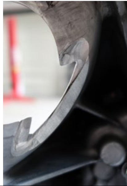
Modified chamfer on the starter pocket from inside bellhousing.
