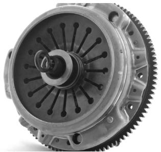
Ensure the friction disc is centrally aligned to the pilot bearing and then tighten in a star pattern in several steps. Finally torque to 25Nm/ 19 ft.lbs.
