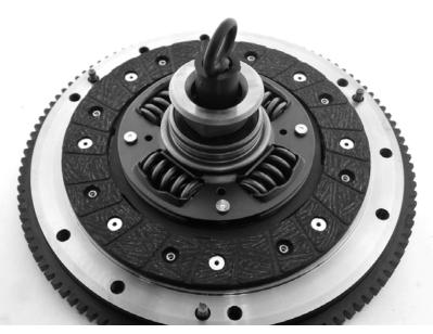
Step 3) Place the pressure plate over the friction disc/ release bearing and loosely mount the pressure plate bolts. The pressure plate will only fit on one orientation way due to the offset dowel location.
