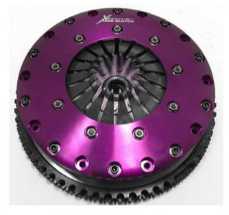
9. Start to do the 10 bolts up ¼ turn at a time in a circular motion. After every rotation remove and re-fit the alignment tool to check the discs are aligned to the pilot bearing.
