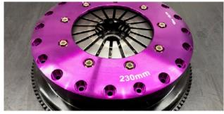
8. Loosely start the threads on 10 of the 20 M6 pressure plate bolts. Use the alignment tool to hold the discs central to the pilot bearing whilst slowly tightening the 10 pressure plate bolts by hand.
