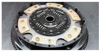
7. Mount the main pressure plate casting into the adapter ring with the fulcrum facing up. Then mount the alloy cover to the adapter ring
