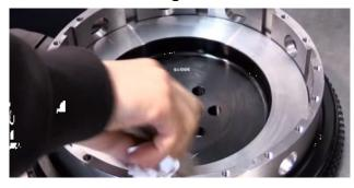
4. Use thread locking compound on the flywheel bolts and torque to manufacturers specifications.
