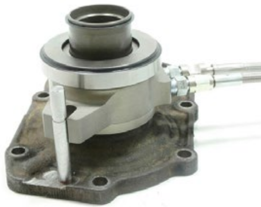
GUIDE PIN FITTED TO NOSE CONE ON R154 TRANSMISSION
