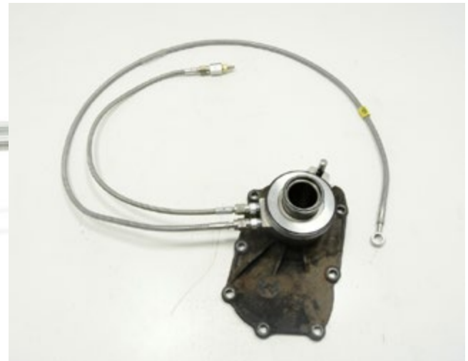
GUIDE PIN FITTED TO NOSE CONE ON R154 TRANSMISSION
