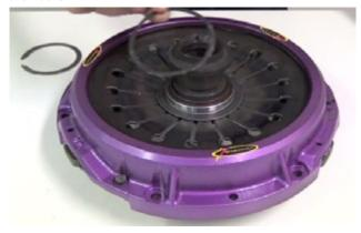
(7) Using C-clip spreaders install the c clip on the bearing to hold in in place against the diaphragm
