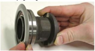
(4) Push down on the bearing and install the C-Clip
