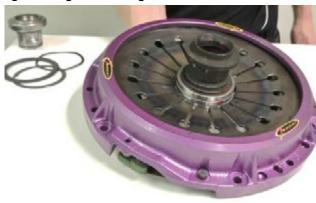
(6) Install the nylon shim on top of the diaphragm followed by the wave washer.
