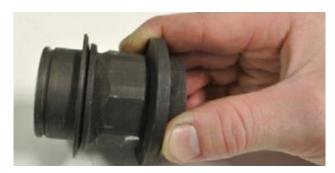
(3) Slide the bearing onto the carrier with the rounded contact face for the diaphragm facing toward the transmission.
