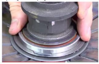
(8) Ensure the transmission is clean and clear of any dirt or old grease. Apply high temperature bearing grease to the nose cone and spline and remove any excess.
