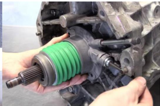
Use thread locking compound on the mounting bolts and torque to the manufacturers specifications.
