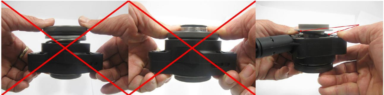
Never spray brake cleaner or solvents in or around the CSC. This can cause the seals to swell and wash away the assembly lubricant.
