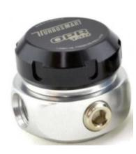
Patent pending OPR T40 is an oil pressure regulation system for turbochargers. It helps prevent compressor or turbine stage oil leaking/smoking and takes the guesswork out of oil restrictor sizing for more efficient and effective oil delivery. The OPR ensures the oil pressure going to the turbocharger never exceeds 40psi, regardless of engine oil pressure. A true plug and play setup for oil feed to turbochargers, restrictors not required.
