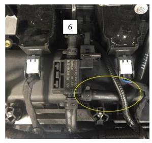
7. Now route the new 5mm ID boost/vac hose alongside of the factory PCV line attaching it with zip ties to hold it in place. You will attach the end of the hose to the hard line under the intake. See photo follow yellow line.
