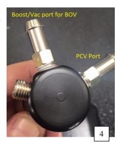
5. Install Boost Reference Adapter on to the PCV fitting on the intake manifold and install the retaining clip. Hook up the PCV with the supplied 130mm PCV hose to the lower fitting, also install the supplied 5mm vacuum hose to the other post as shown below. Use slotted hose clamp and spring clamp to secure each hose in place respectively.
