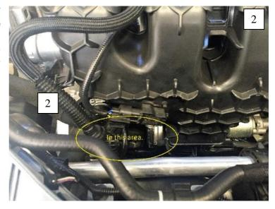
Cut the OEM hard line tubing off the quick connect fitting by slicing down the tube in various positions and the fitting should fall out. Take care not to cause personal injury. Repeat for the PCV end of this line.
