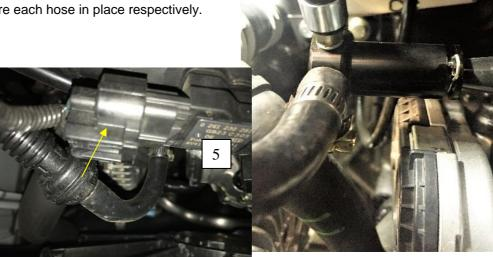
6. On the BOV control valve, remove the following line marked in the photo from the valve and the hard line under the intake. Cap the BOV control valve with the supplied vacuum cap.
