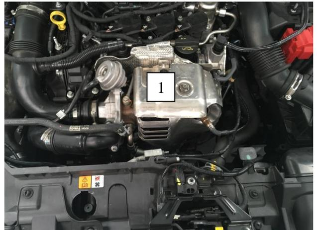
2. Remove charge pipe outlet secured by 2x 10mm nuts and hose clamp.
