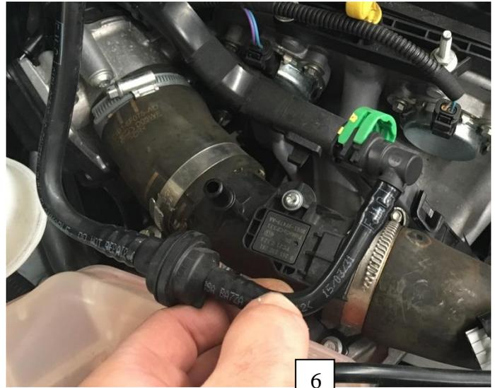
7. Cut the OEM hardline tubing off the quick connect fitting by slicing down the tube in various positions and the fitting should fall out. Take care not to cause personal injury. Repeat for the PCV end of this line.
